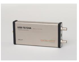
The Signal Hound TG124A is a USB-powered, 100 KHz to 12.4 GHz, economy tracking generator and CW signal generator. The TG124A turns your SA124B, SA44B, or BB60C spectrum analyzer into a versatile scaler network analyzer. The combination can measure gain, frequency response, compression, flatness, and insertion loss on components and subsystems.
